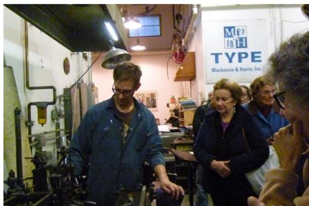
An M & H typesetter melts together lead, tin, and antimony, used to cast type. M & H, adjacent to Arion Press, is the largest type foundry in North America, and one of the largest in the world.
